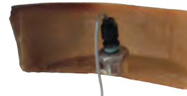
Assemble with 4" from bushing top to end of sensor
