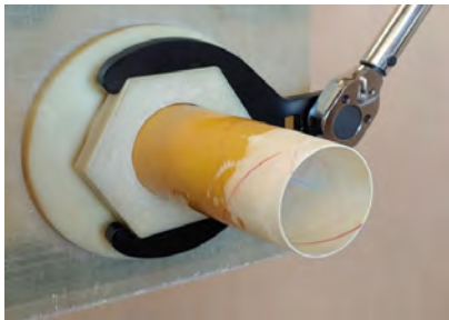
Tightening Compression Nut for NOV Pipe
